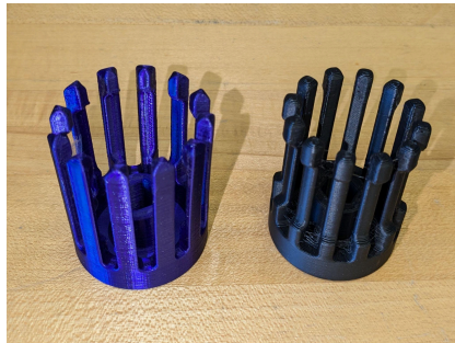
FIGURE 1. Spline coupling with radially tapered fingers.
